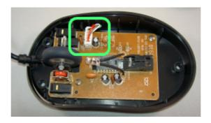
This connector inside the mouse will be disconnected as this cable will be connected to the USB hub. To connect the cable to the USB hub the wires will be cut and then soldered to the PCB of the USB hub.
